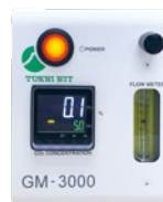
CO2 Gas Mixing Unit
